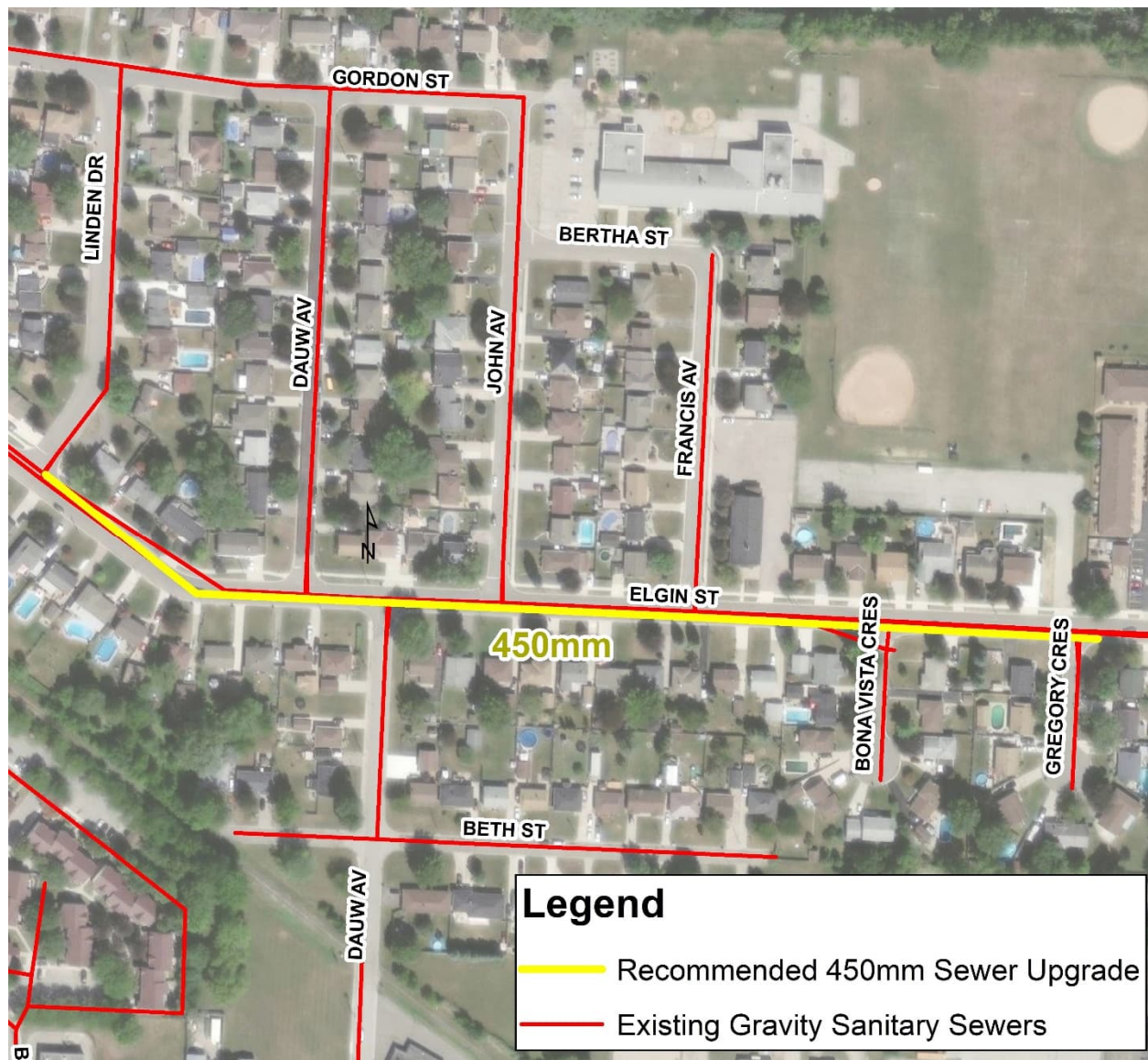
Figure 10-10: Wallaceburg Sewer Upsizing to Address Capacity
