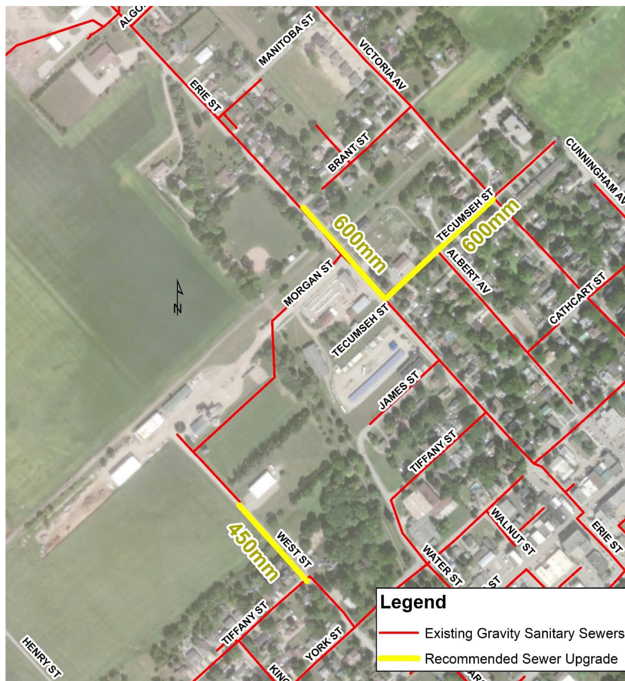
Figure 10-8: Ridgetown Sewer Upsizing to Address Capacity
