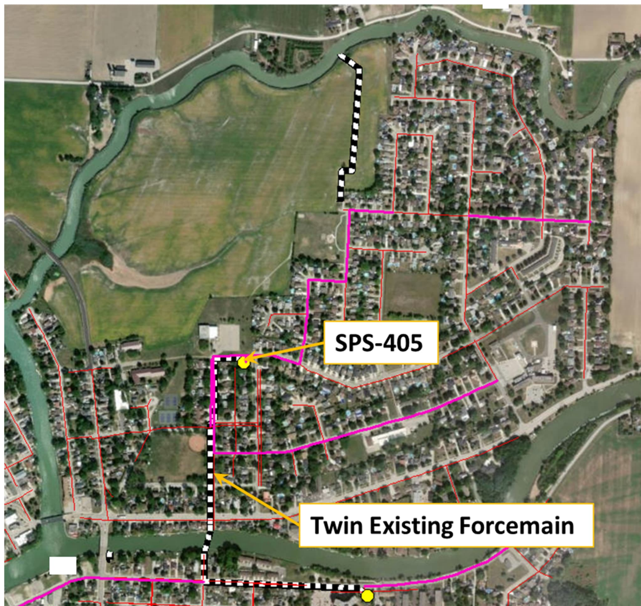
Figure 10-16: Pump Station Upgrade to Wallaceburg SPS-405
