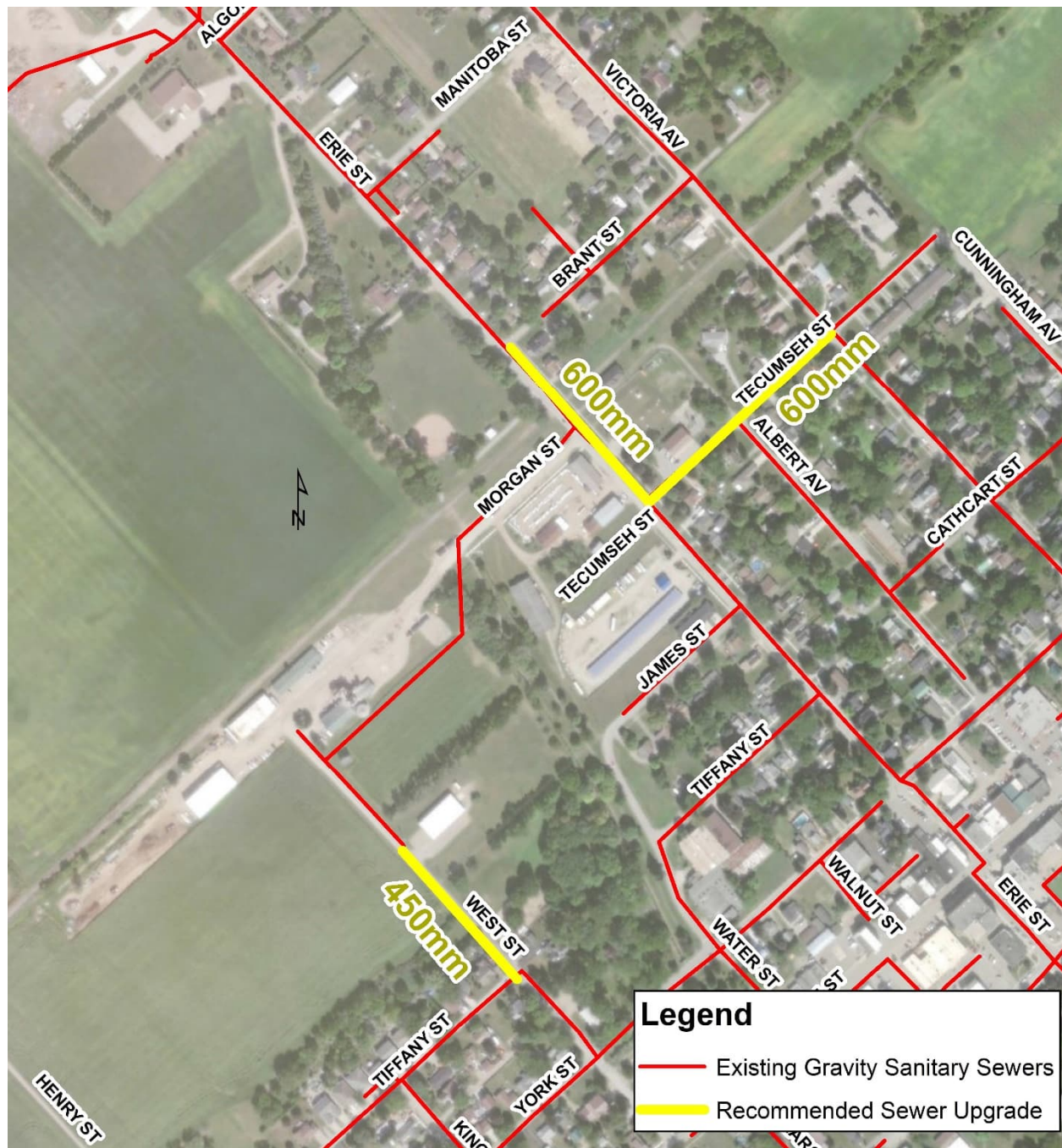
Figure 10-8: Ridgetown Sewer Upsizing to Address Capacity
