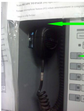
To operate the microphone hold down the button on the side hold. Hold it 8 – 10 inches from your mouth and speak clearly and slowly. When you are done speaking release the button on the side. (Any time the button is held down the microphone is operational and the entire building can hear what you are saying!)
