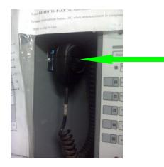
To operate the microphone press the button on the side hold, wait for the tone to stop, hold the microphone 8 - 10 inches from your mouth and speak clearly and slowly. When you are done speaking release the button on the side. (Any time the button is held down the microphone is operational and the entire building can hear what you are saying!)
