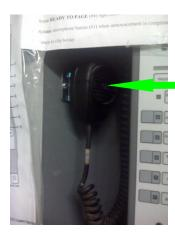
To operate the microphone press the button on the side hold, wait for the tone to stop, hold the microphone 8 – 10 inches from your mouth and speak clearly and slowly. When you are done speaking release the button on the side. (Any time the button is held down the microphone is operational and the entire building can hear what you are saying!)
